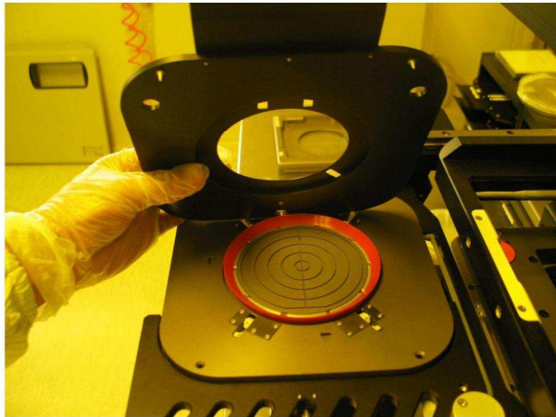
15.將有模仁(stamp)的試片反過來放好(圖向下),按 countiune
