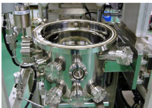
Stainless steel chamber with multiple spare ports allows the use of multiple analytical instruments.
